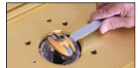
Marc's ingenious bent Collet Wrenches let you change bits fast without changing router height
